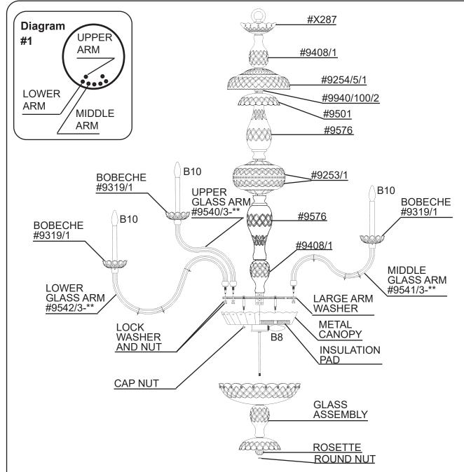
6 Install arms into large arm washer. Line up holes in arms with dimple in washer. Use lock washer and nut to secure arms in place. NOTE: Place 8 upper arms into inside diameter holes and ALTERNATE 16 middle and lower arms in outside diameter holes. For best appearance line-up lower arms with upper arms. See Diagram #1.
