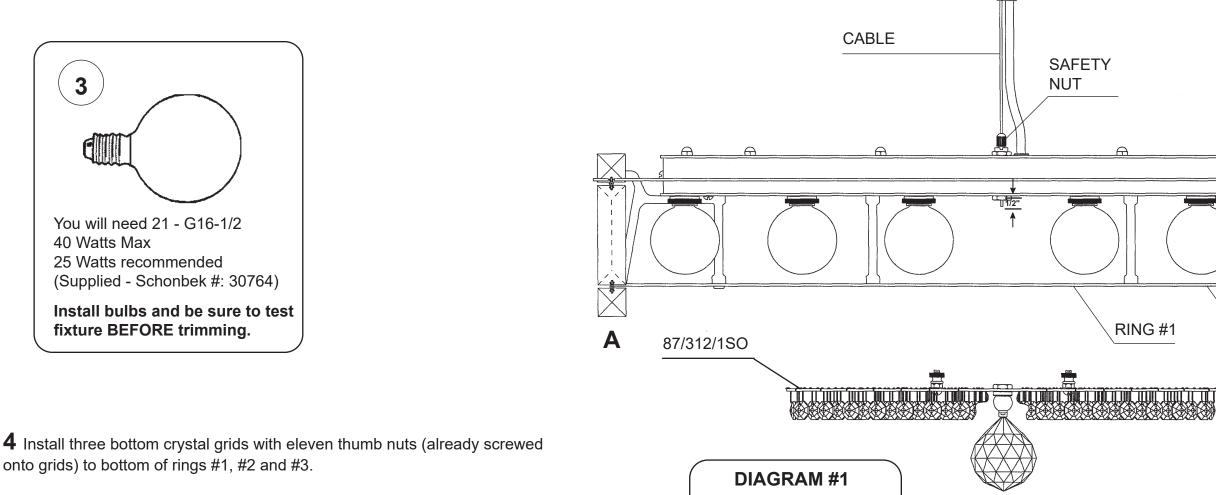
**5** Screw ball "B" onto bottom of grid 87/312/1SO. Tighten set screw to lock into position. (Diagram #1)
