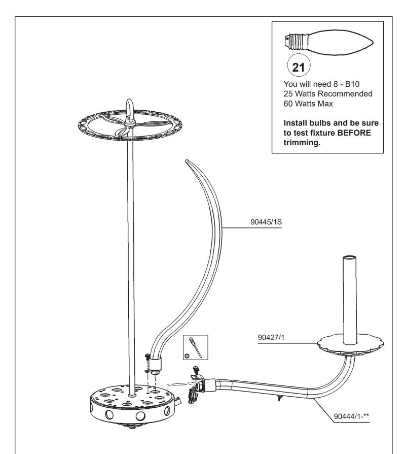
19 Connect arm wires using plug-in connectors. See detailed illustration.
