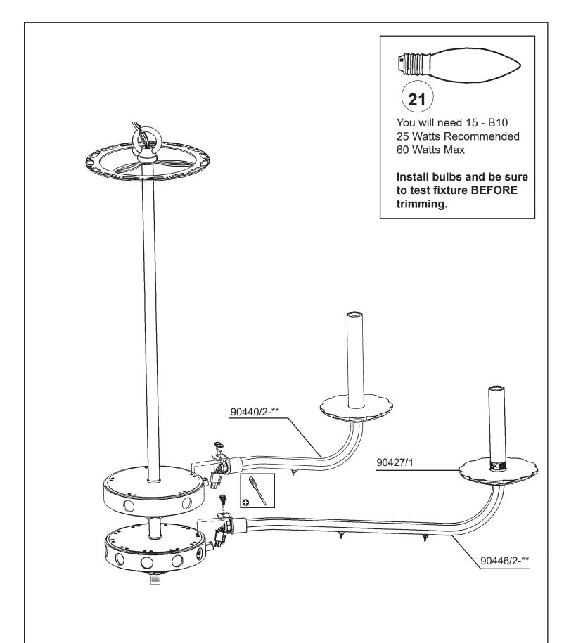
19 Connect arm wires using plug-in connectors on top and bottom tiers. See detailed illustration.
