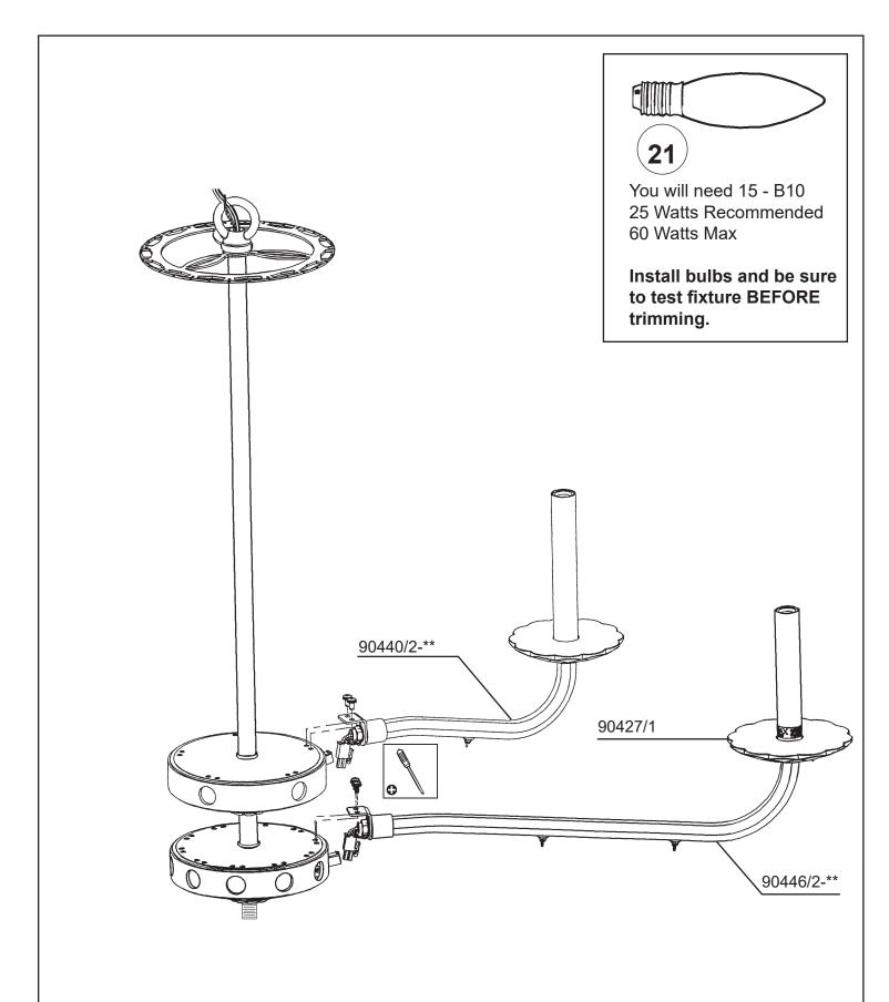
19 Connect arm wires using plug-in connectors on top and bottom tiers. See detailed illustration.
