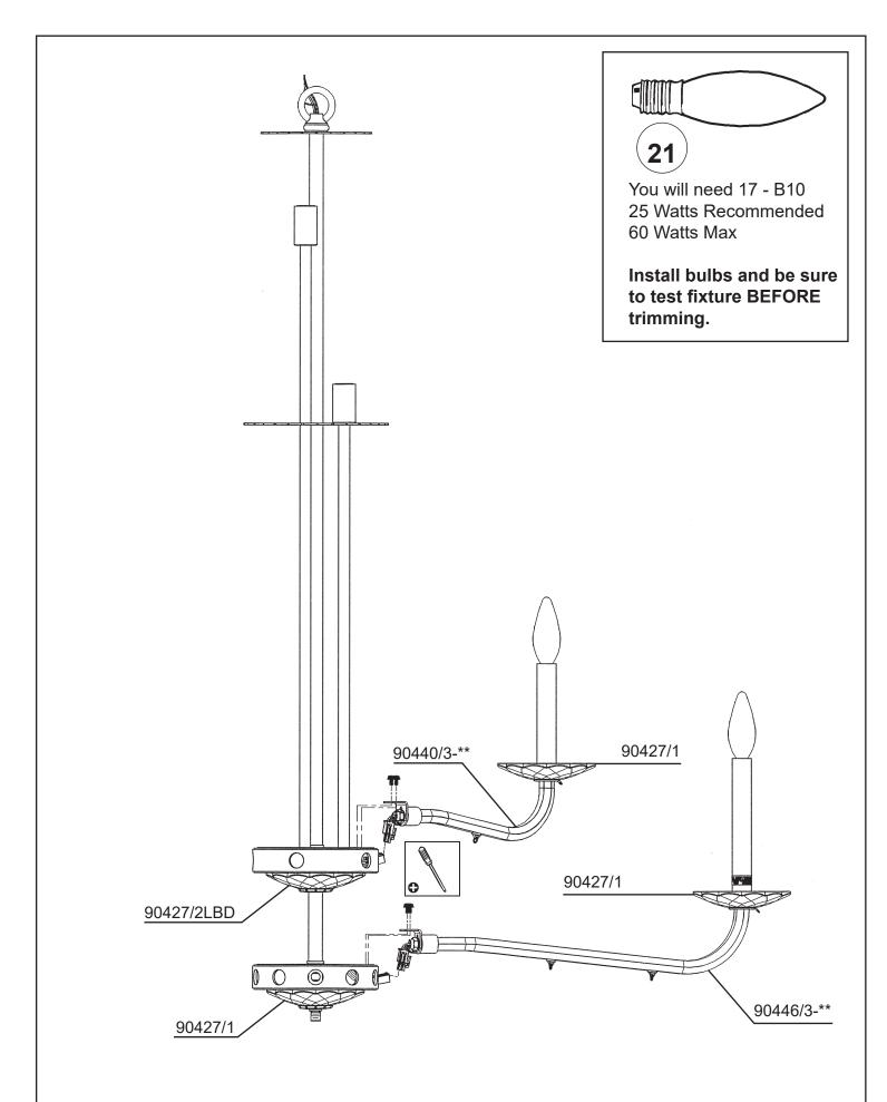
19 Connect arm wires using plug-in connectors. See detailed illustration.
